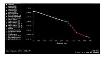
For the third orientation the insulator is avoided and then it was analysed and the temperature drop in PCM layer is found to be around 1°C which is having the least temperature drop. The graph is shown below,
