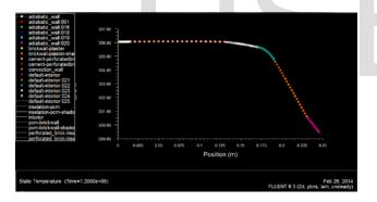
For the second orientation where the PCM is placed left to the insulator the temperature drop across the PCM is found to be 1.4°C which can be somehow give out the needed efficiency.
